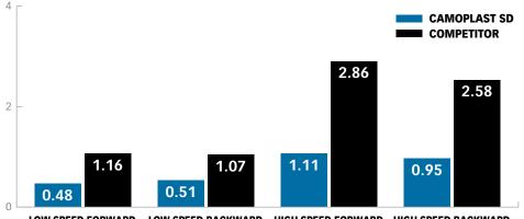
Throughout the entire test, the vibration level was 60% lower with the Camoplast tracks than a OEM quality track regardless the speed and the direction.
