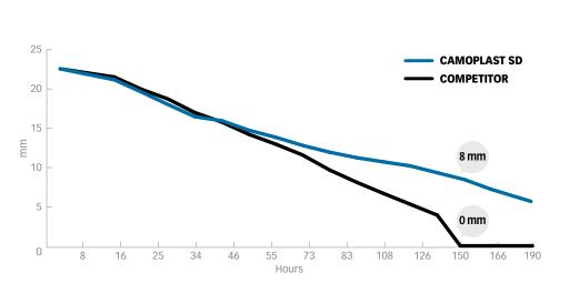
In this test, we clearly see that the competitor track tread compound was wearing faster versus Camoplast. Maintaining more rubber around the carcass offers more protection and translates in longer service life. The end result is: Camoplast SD offers 20% more service life.
